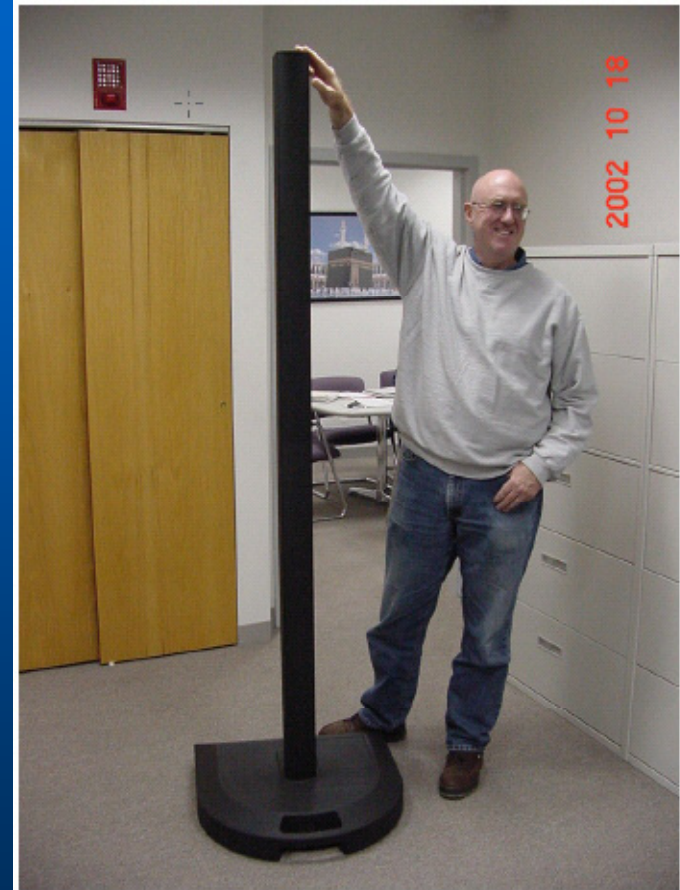
The final prototype of the Cylindrical Radiator loudspeaker is shown (with inventor Clifford Henricksen).
